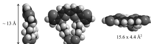
Figure 6. Molecular structure of dithiol 2 drawn from ellipsometry data in a conformation favorable to double fixation on gold (from MOPAC-ChemDraw 3D optimization).
